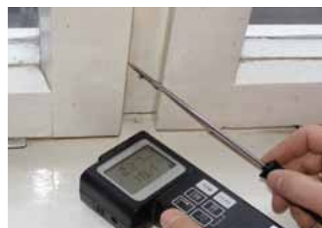
Testing on wind speed, thermoanemometer
